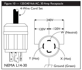
This receptacle powers 120/240 Volt AC, 60 Hz, single phase loads requiring up to 2,775 watts of power at 23.1 Amps for 120 Volts; 5,550 watts of power (5.55 kW) at 23.1 Amps for 240 Volts. The outlet is protected by a push—to—reset circuit breaker.
